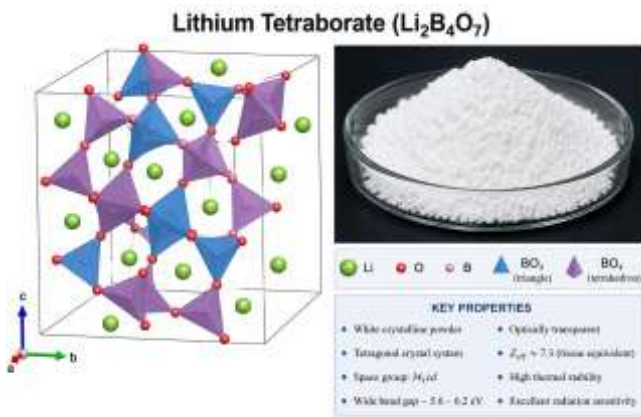
Figure 1. Crystal structure and key characteristics of lithium tetraborate ( \text{Li}_2\text{B}_4\text{O}_7 ).
